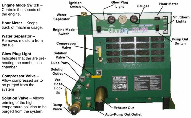
Solution Outlet – Hook up for the 3/16" solution hose
