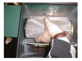
3. Clean the stainless steel filter of debris **daily**. This filter is
