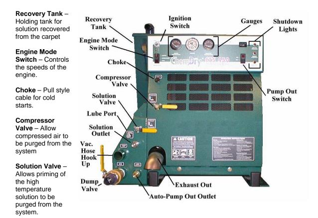
Solution Outlet - Hook up for the 3/16" solution hose
