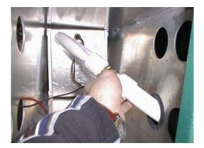
5. Remove automatic pump out filter screens and clean.
