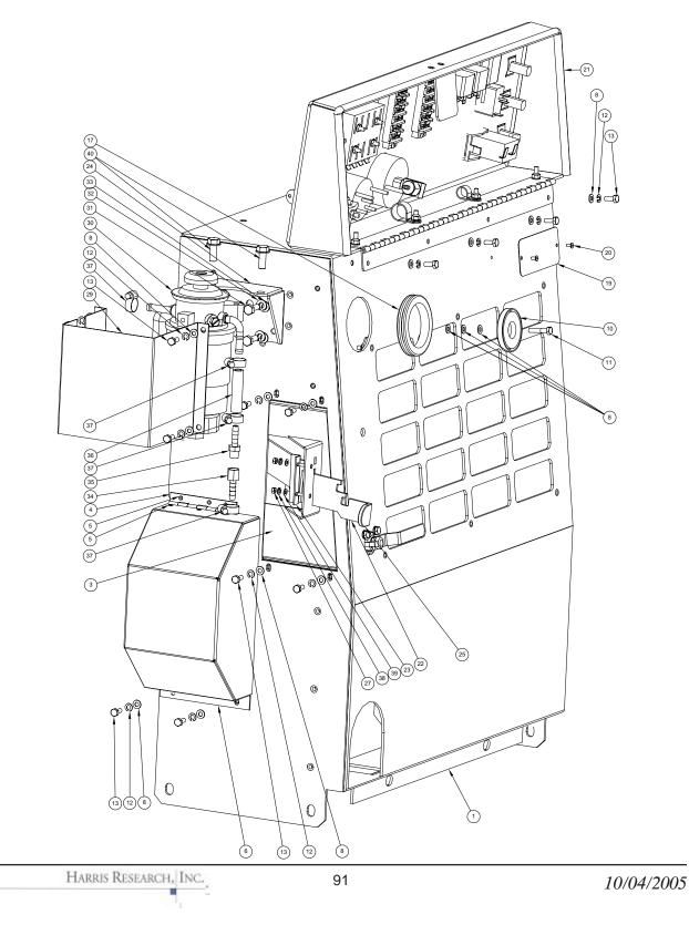
Figure 34 Dash Assembly CTS 450 Diesel - Rear View D-5867 Rev B
