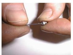
4. Re-install filters and orifices.
