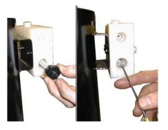
Clean the filters and orifices with fresh water or compressed air.
